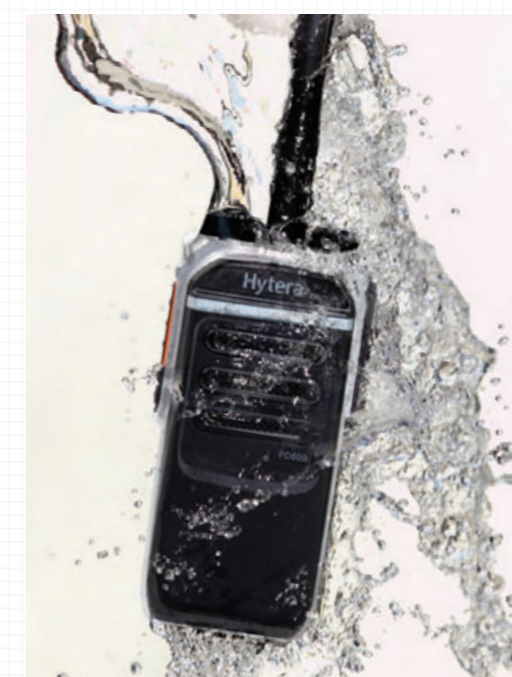
Both new models are built for ruggedness and reliability, meeting MIL-STD 810 c/d/e/f/g. On top of this, the PD60X (seen here undergoing a soaking) is IP67 rated, withstanding immersion in water one metre deep for at least 30 minutes. To its left is the PD50X, a basic DMR radio offering dual-mode (analogue/digital) communication, long battery life (over 16 hours in typical use) and light weight (260g)
